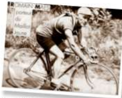
Steel frame One Gear – fixed wheel Brakes – Wooden wheel rims Drop Handlebars
